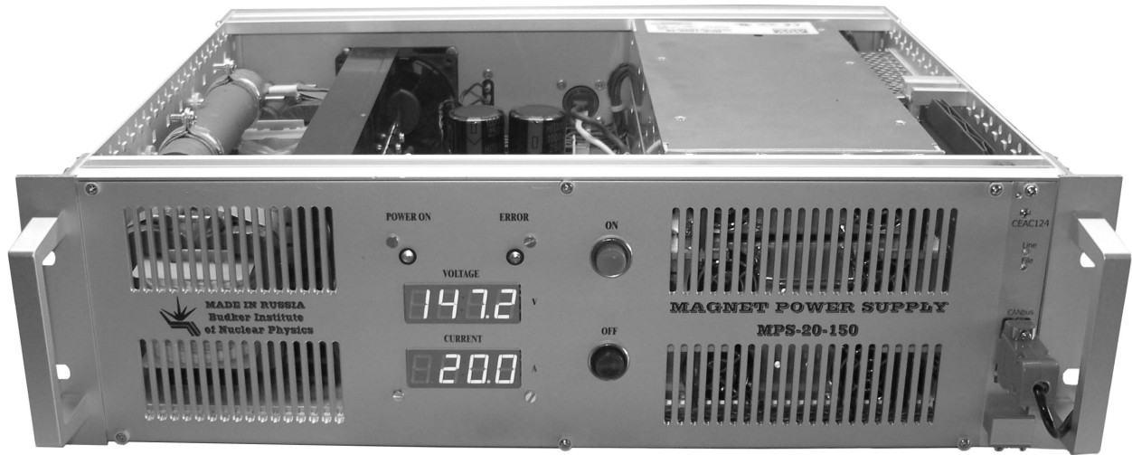
Figure 4: Magnet power supply MPS-20
