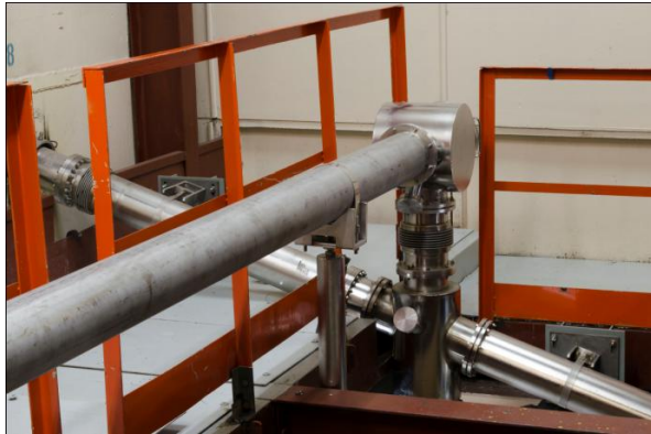
Figure 7: Optical beamlines for the first and the second stage FELs. Radiation of both FELs is delivered to the same user stations. Switching between FELs is done by retractable mirror.
