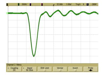
Figure 4: Modulator output pulse on 25  $\Omega$  load
