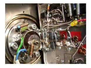
Figure 5: Cathode-grid unit and modulator.
