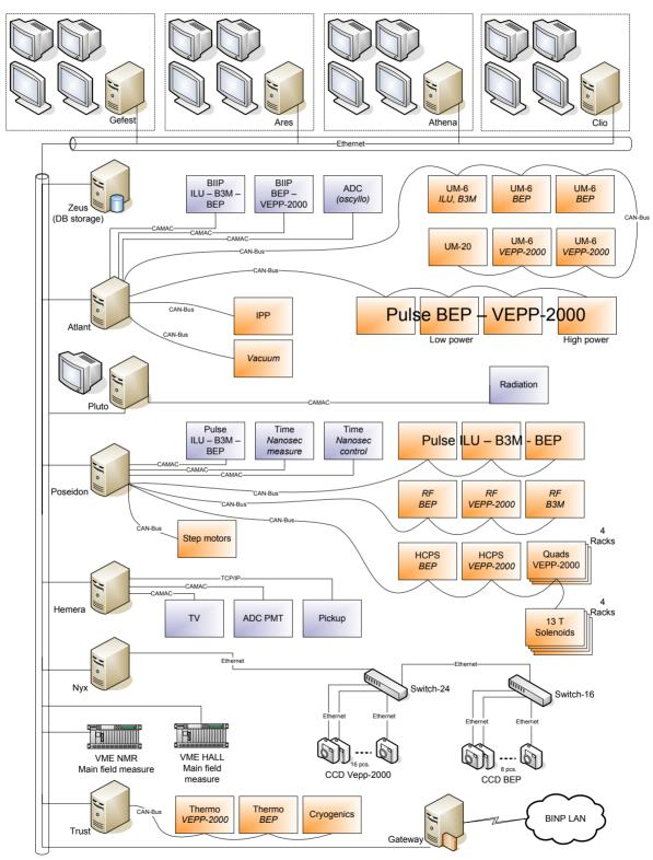
Figure 2: Hardware of VEPP-2000 Complex automation system.
