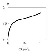
Fig.3. A decrease in  $\alpha$  as a function of  $\omega L_1/R_H$ .
