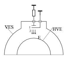
Fig.6. Schematic diagram of the rotor voltmeter operation principle.
