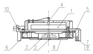
Fig. 7. General view of the rotor voltmeter.
