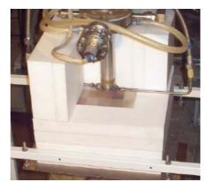
Figure 2: Epithermal neutron beam shaping assembly (disassembled in part).
