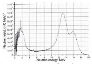
Figure 4: Neutron spectra from  ${}^{7}\text{Li}(d,n)2^{4}\text{He}$  reaction measured by time of flight method.
