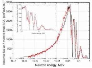
Figure 3: Measurements (dots) and calculation (line) epithermal neutron spectra from BSA
