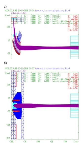
Figure 6: The ion beam transportation through the low energy beam line, 1-st stage of tandem acceleration and stripping target.
