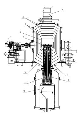
Figure 1: Scheme of the VITA facility. 1-ion source (H<sup>-</sup>); 2 – high voltage electrode; 3 – electrode shutters; 4 – cryo pump; 5 – accelerator vacuum volume; 6 – intermediate electrodes; 7 - stripping target; 8 - feedthrough insulator (vacuum part); 9 – feedthrough insulator (gas part); 10 – high voltage source; 11 – coaxial feeding tubes.
