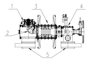
Figure 3: The new injector for BNCT facility:  $1 - H^{-}$  ion source; 2 – bending and focusing magnet; 3 – accelerating tube; 4 – beam diagnostics; 5 – valves for turbomolecular pumps.
