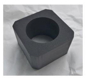
Fig. 6. Sintered B<sub>4</sub>C block made by Virial.
