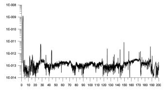
Fig. 3. RGA scan at 100  $^{\circ}$ C for the same ceramics after one year in vacuum (at room temperature).
