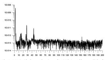
Fig. 2. RGA (residual gas analyzer) scan for Virial-sintered boron carbide after 24 h at 100  $^\circ\text{C}.$
