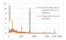
**Fig. 9.** Gamma-ray spectrum of SS 316L-IG after 28 min after the end of neutron generation (the sample is placed at a distance of 50 cm from the detector) and after 3 days (the sample is placed close to the detector).
