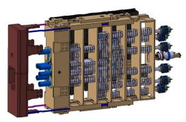
**Fig. 5.** Typical EP#11 Port Plug DSM Assembly (left – two DFW, center – DSM frame and vertical plates with diagnostics, the back side shows trays with ceramics (Figs. 4 and 5)).
