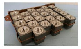
Fig. 7. BINP made full scale mockup of shielding tray with hot-pressed blocks made by NEVZ.
