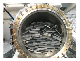
Fig. 1. 638 bars of sintered ceramics inside high vacuum test-bench before measurements. Ceramics produced by Virial. Total surface area of samples is  $4.56 \text{ m}^2$ .
