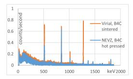
Fig. 8. Gamma-ray spectrum of two samples of boron carbide ceramics after activation of fast neutrons.
