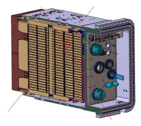
**Fig. 4.** EP#11 integrated Port Plug. Inside the port plug structure (PPS) there are DSM modules. Port plug section between first and second DSMs is shown.
