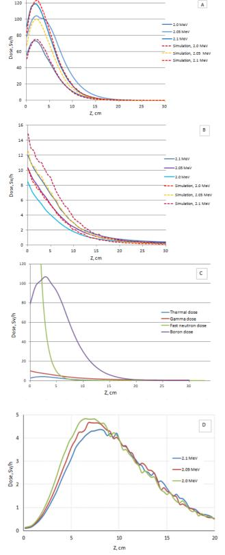
Figure 2: boron dose (a),  $\gamma$ -dose (b), the distribution of all doses along the beam axis (c), the ratio of the "useful" to "harmful" dose (d).
