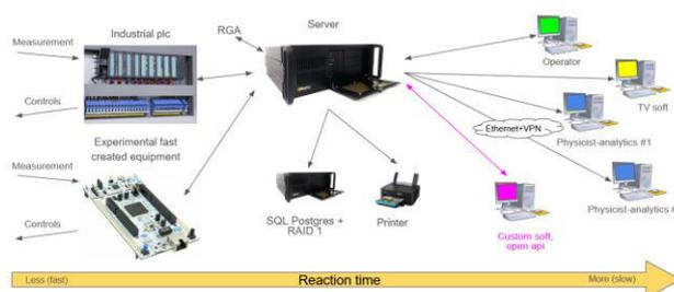
Figure 1: System architecture.
