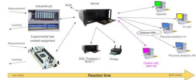
Figure 1: System architecture.
