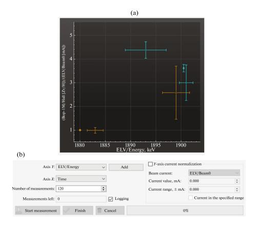
Fig. 4. Dependency building panel: (a) dependence of the readings of the gamma detector (divided by the beam current) on the beam energy; (b) settings panel.
