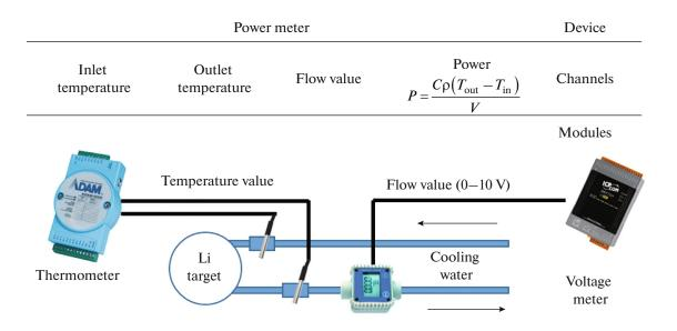
Fig. 2. Server architecture using the example of a power meter.
