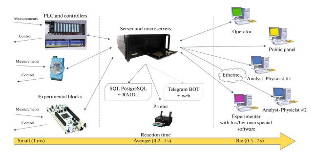
Fig. 1. Architecture of the developed automation system.
