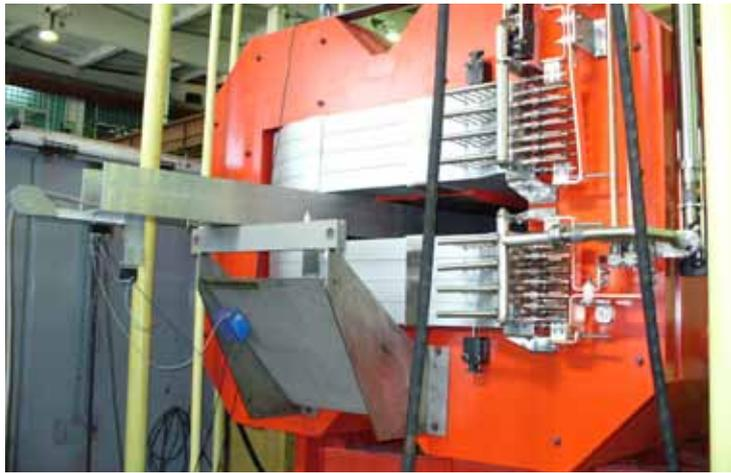
Fig.(6.4)2. Radiation-resistant dipole magnet at the bench for magnetic measurements.
