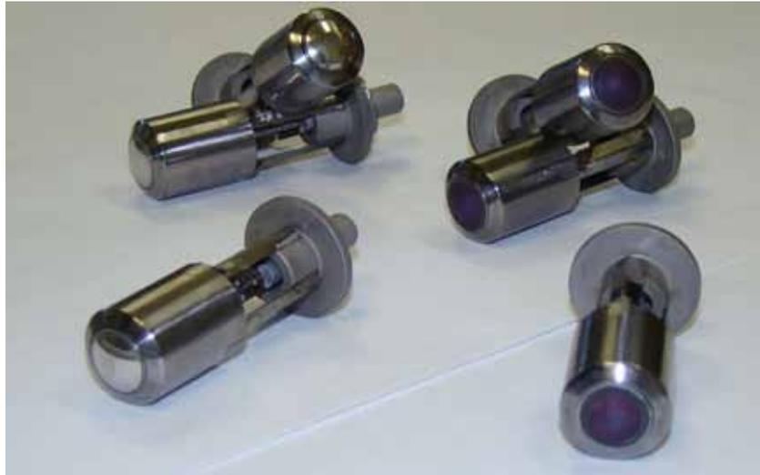
Fig. (5.6)1. General view of the cathodes for BNL (USA).
