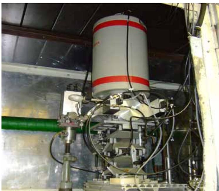
Fig.(6.1)31. 9-element detector made by Canberra on beamline 8 (the EXAFS spectroscopy station).
