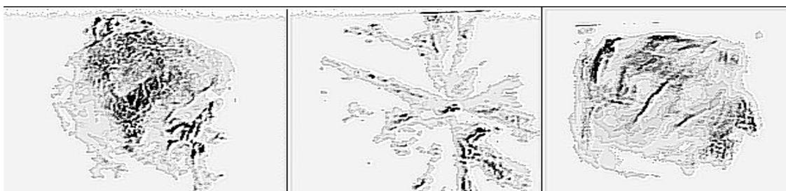
Fig.(6.1)24. Topographs of diamond of different morphology made in reflected radiation.
