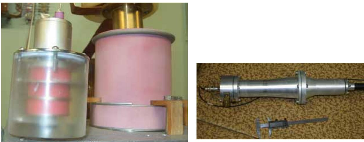
Fig.(5.14)1. Thyratrons TPI1-1k/35 and TGI1000/25 and a 50 ohm load (from left to right).
