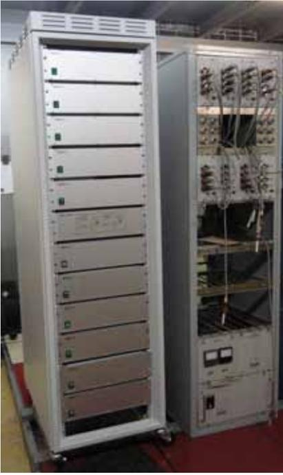
Fig. (5.3)9. New rack of ion pumps power supplies.
