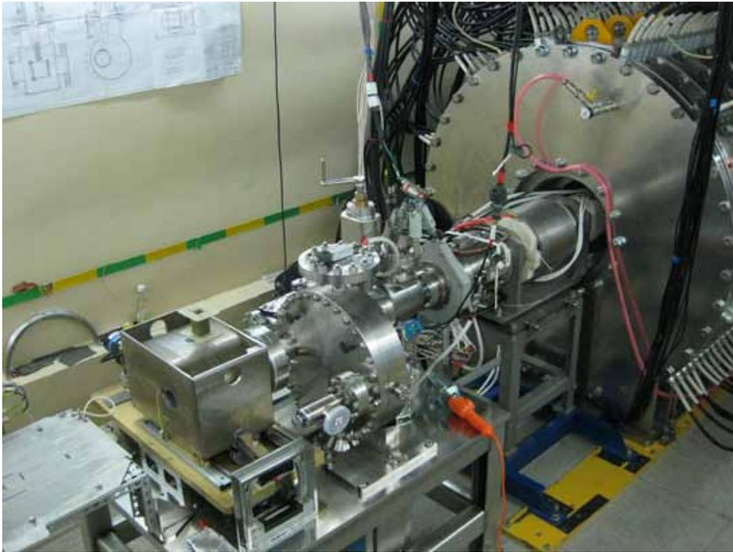
Fig. (5.4)2. Accelerator target assembly and front part of accelerator.
