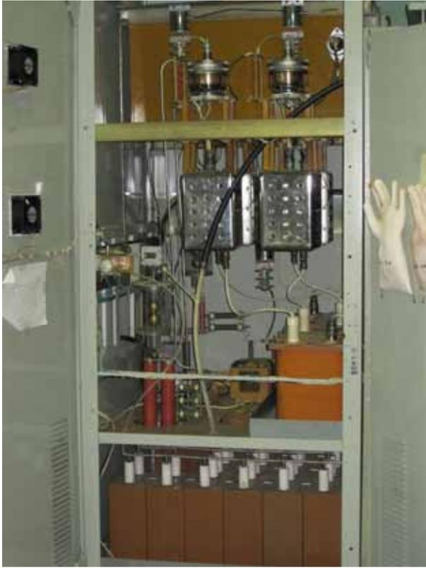
Fig.(5.11)3. Anode modulator.
