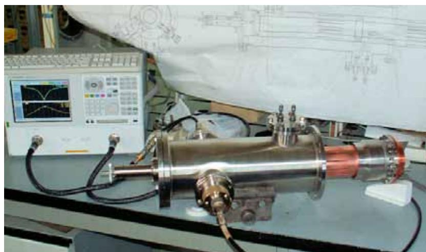
Fig.(7.5)4. Source of electrons at the measurement stand.
