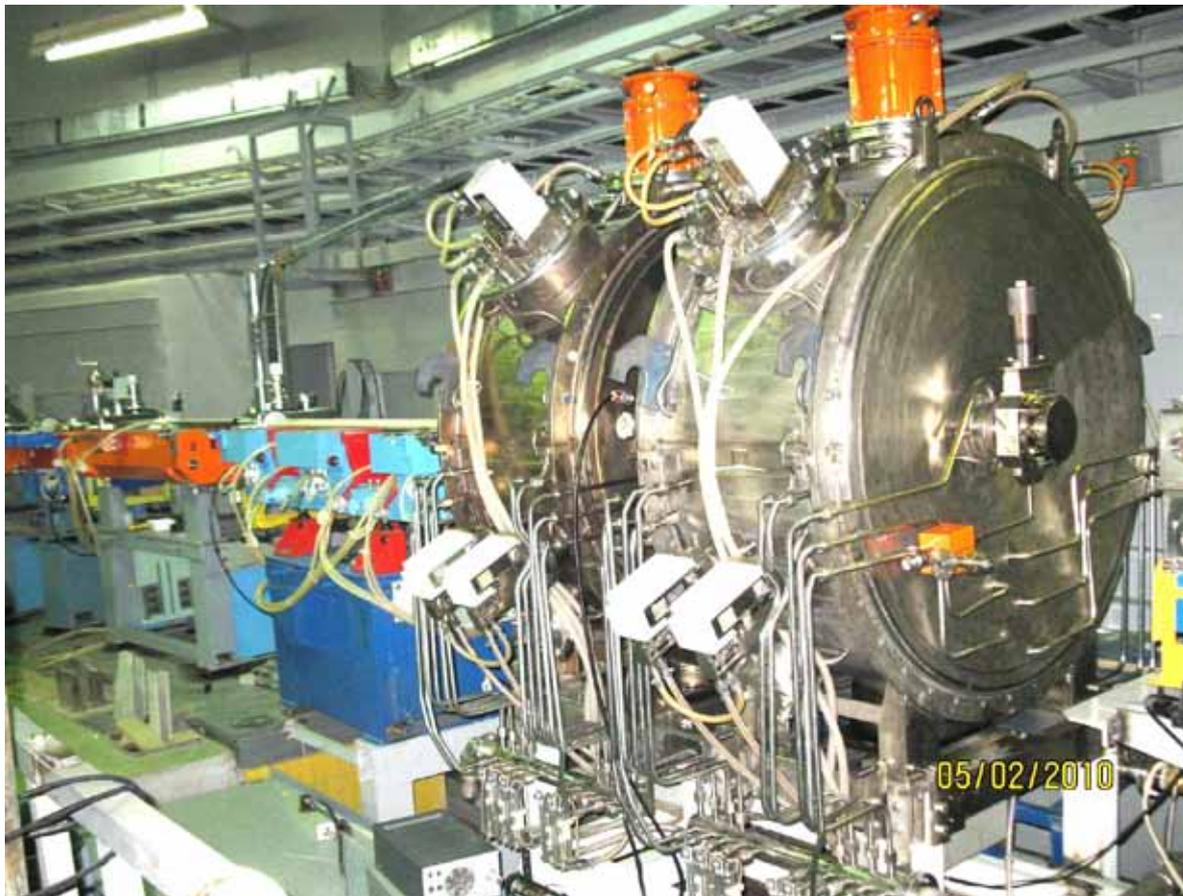
Fig.(7.9)1. Two accelerating cavities in the 2.2 GeV storage ring.
