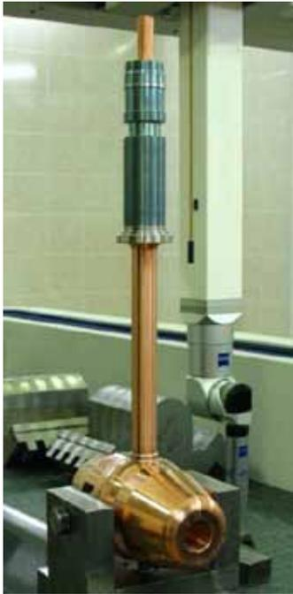
Fig.(7.13)2. Pilot sample of the drift tube.
