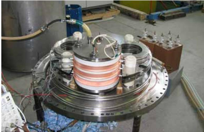
Fig.(5.7)2. Transformer section under testing.
