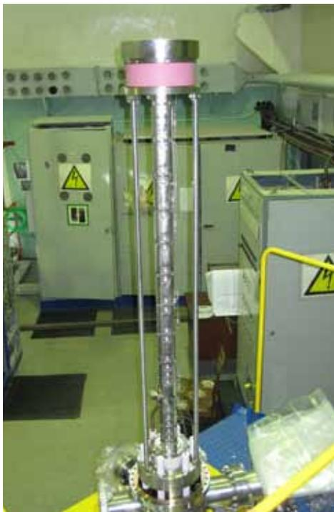
Fig.(5.11)1. Drift structure of MIS-1.
