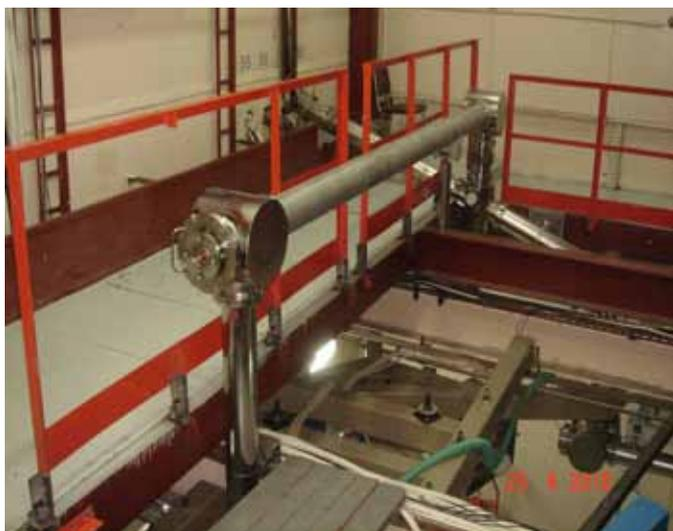
Fig.(6.3)22. Radiation extraction beamline of the second stage FEL (middle part). Radiation coming from below is reflected from two mirrors and gets into the “old” part of the beamline (in a distance) through the movable mirror assembly.
