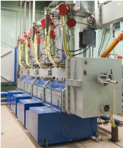
Fig. 7.6.1. 4-module output stage of the generator with self-excitation suppressors installed.
