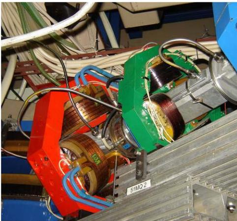
Fig. 6.4.2. Quadrupole lenses in achromatic bend.
