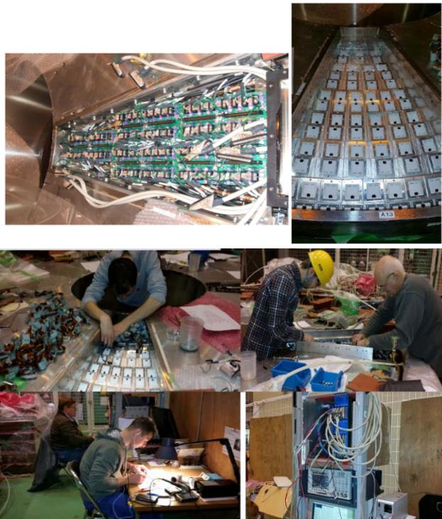
Fig. 1.8.8. Stages of disassembly of sector of calorimeter and replacement of resistors.
