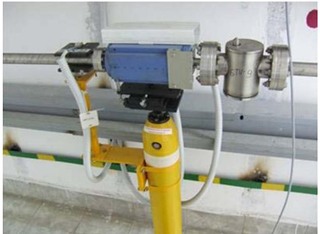
Fig. 5.1.3. K-500 unit: dipole corrector, quadrupole, luminophore probe.
