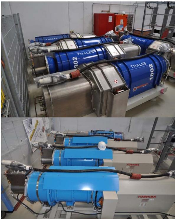
Fig. 5.6.3. Storage of tested klystrons with Connection Modules before their installation in tunnel of XFEL.
