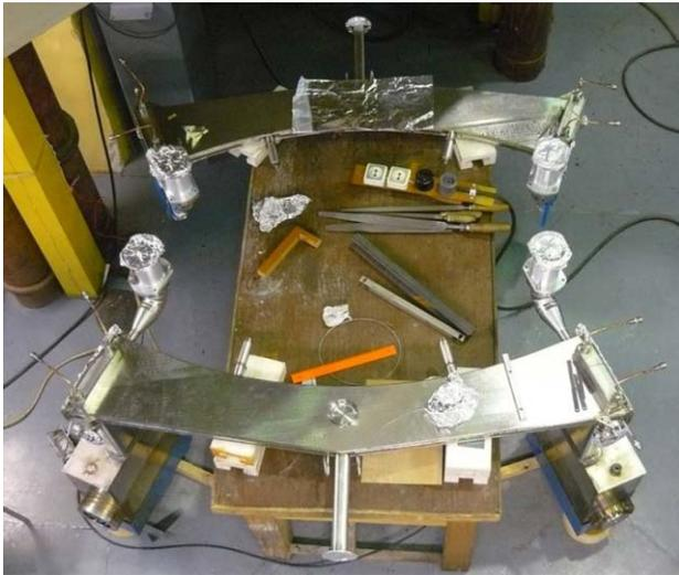
Fig. 5.1.13. New vacuum chambers with additional inflector plates.
