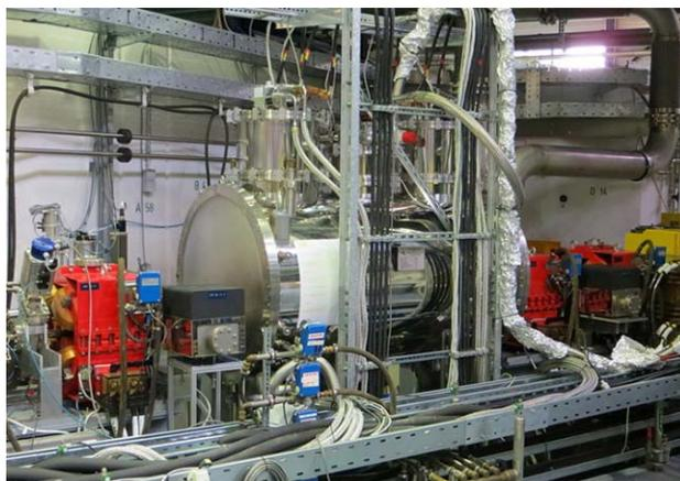
Fig. 6.5.1. 40-pole wiggler with field of 2.5 T and a period of 48 mm installed on ANKA storage ring (Karlsruhe, Germany) for research in spectroscopy.
