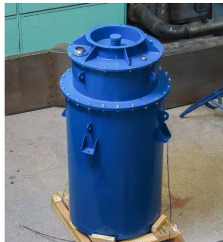
Fig. 6.4.3. New high-voltage rectifier for electrostatic electron gun.
