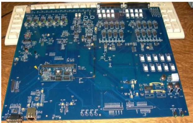
Fig. 7.1.1. Photo of PCB of controller of NICA booster RF stations.
