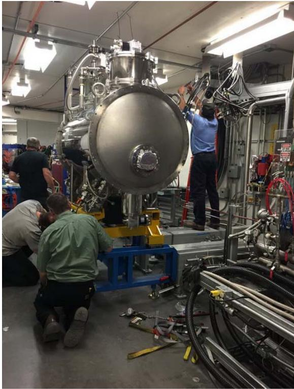
Fig. 6.5.2. Installation of upgraded 27-pole 4 T wiggler BMIT on CLS storage ring (Canada).
