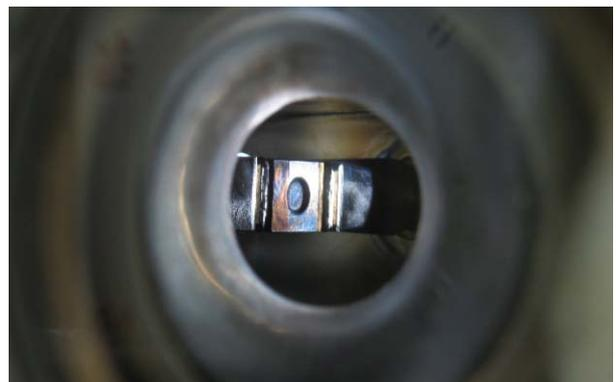
Fig. 5.7.2. Target with ceramic windows.
