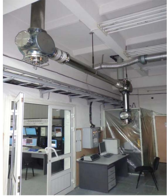
Fig. 6.4.5. Radiation extraction to the second floor. Vessels comprising mirrors are connected by pipes and have adjustment units.
