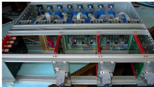
Fig. 7.1.9. Stand for testing of MPS-10 and MPS-5 sources.
