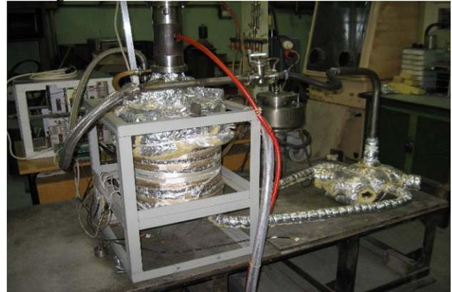
Fig. 5.7.1. Stand for liquid-metal positron target.
