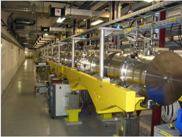
Fig. 7.7.2. CCDTL modules in Linac4 tunnel.
