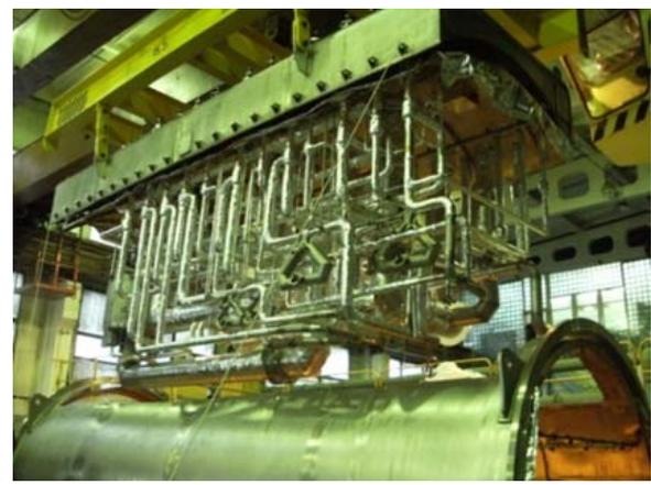
Fig. 5.10.3 Mounting of cold mass of distribution box XLVB in casing. Casing diameter: 2.5m. Casing length: over 7m. Total weight: about 20 tons.
