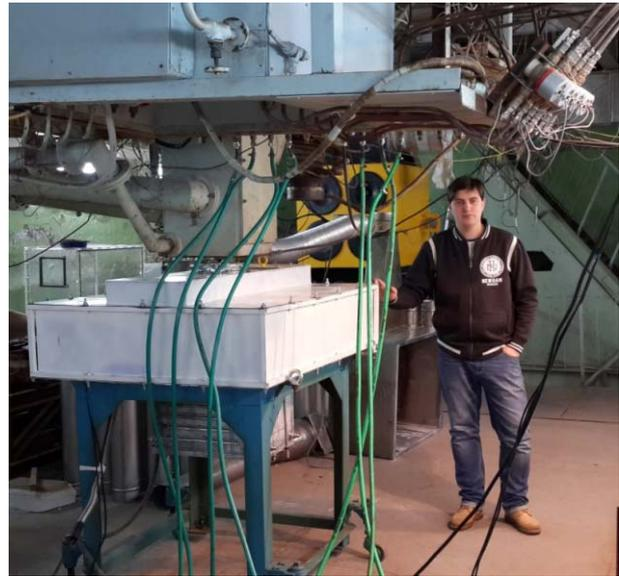
Fig. 8.4.10. Installation for anticorrosion alloying surfacing of Ta based on the titanium alloy.
