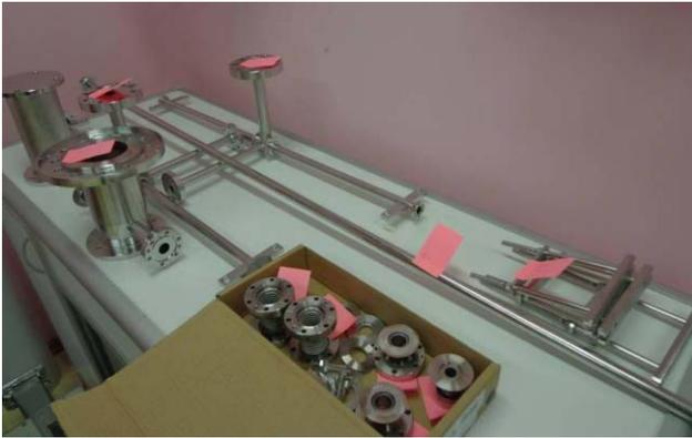
Fig. 5.3.12. Elements of vacuum system of plasma section.
