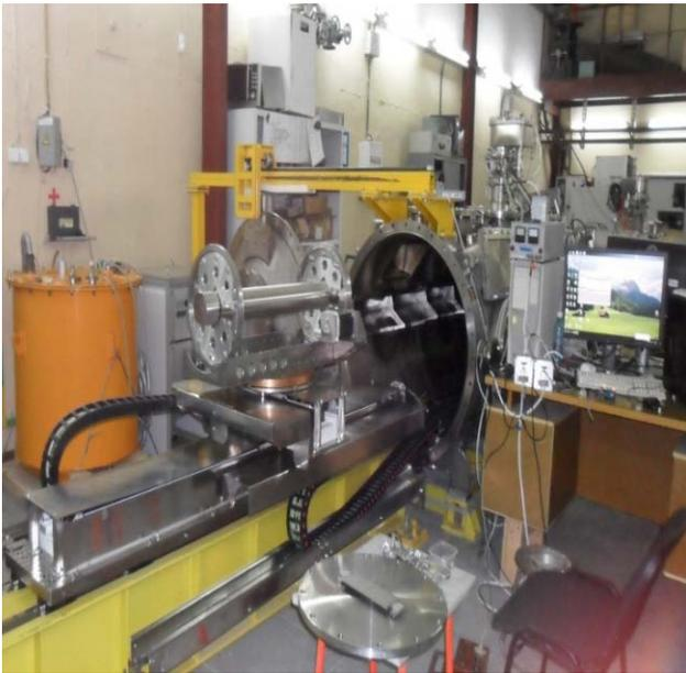
Fig. 5.5.1. Electron-beam welder. Foreground: mechanism for moving part to weld.
