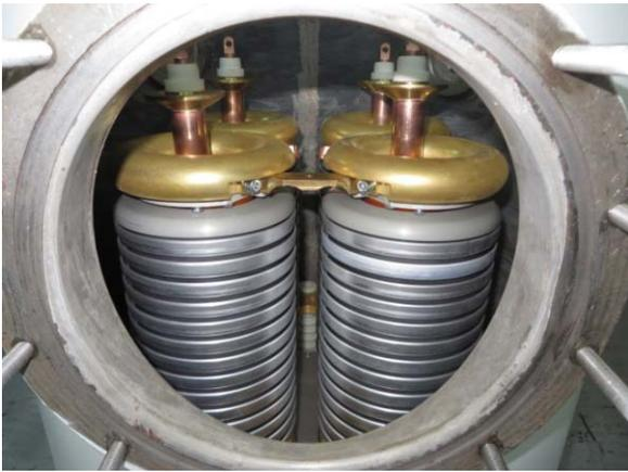
Fig. 7.3.1. Insulating transformer in vessel. View from window for power output.
