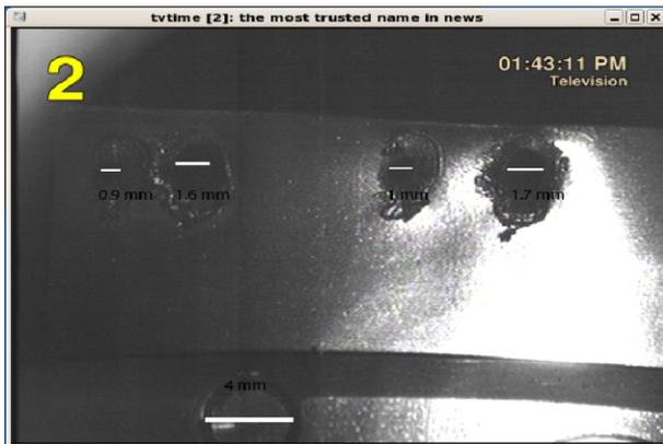
Fig. 5.4.7. Holes burnt by electron beam with correction system switched off.
