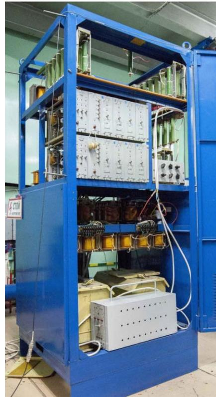
Fig. 7.6.3. Cabinet for low-voltage power supplies with rectifier of bias voltage boost (bottom).
