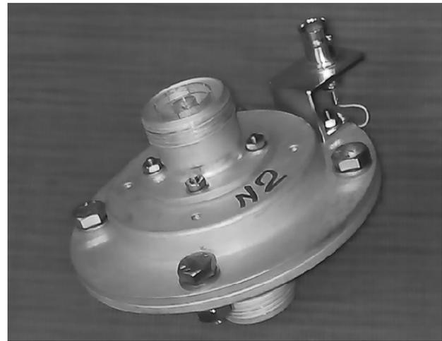
Fig. 5.3.8. Coaxial microwave switch.
