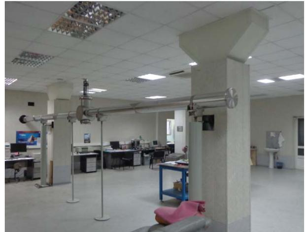
Fig. 6.4.6. Horizontal distribution beam line in hall intended for new user stations.
