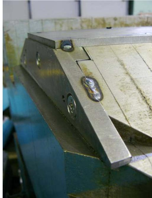
Fig. 5.1.5. Plates on the BEP magnet' pole.
