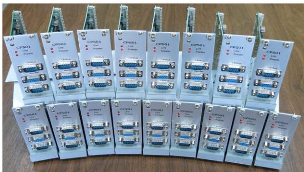
Fig.7.1.8. First serial controllers.
