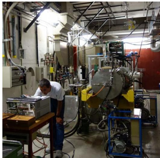
Fig. 7.4.1. Preparation of CCDTL module for tests in shielded hatch, CERN.
