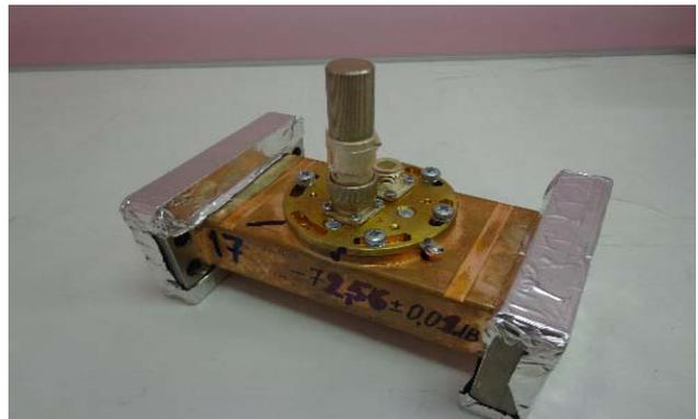
Fig. 5.3.4. Directional waveguide coupler.
