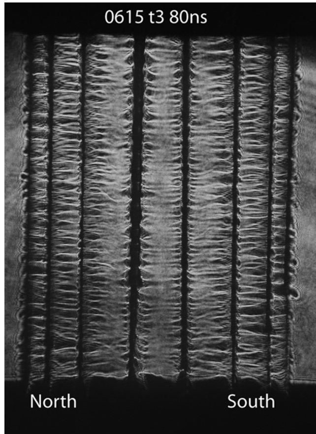
18 19 Figure 3.9. Laser Shadowgraph image of an exploding wire z-pinch on the 1 MA COBRA 20 generator at Cornell that started out with a cylindrical array of 8 12.7 \mu\text{m} Al wires at a radius of 8 21 mm. The anode (cathode) of the array is at the top (bottom). Notice the short wavelength 22 structure in the plasmas around each exploding wire. Also, note that there is a plasma forming 23 on the array axis. Courtesy of the Laboratory of Plasma Studies, Cornell University.
