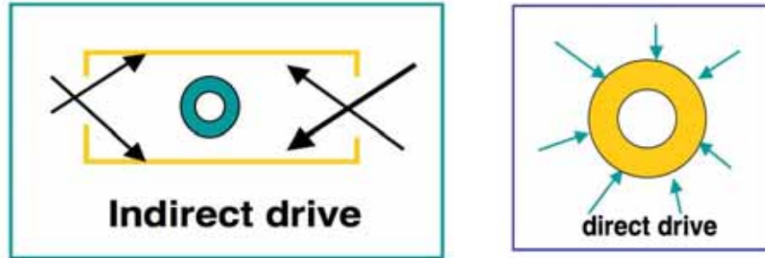
Figure 3.2. Schematic diagrams of the indirect drive and direct drive versions of ICF.
