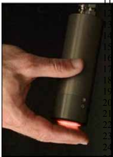
11 12 13 14 15 16 17 18 19 20 21 22 23 24 25 26 27 28 29 30 Figure 2.5.1. The control of atmospheric pressure plasmas provide the ability to economically treat complex surfaces, up to and including living tissue. Courtesy R. Hicks, University of California at Los Angeles.
