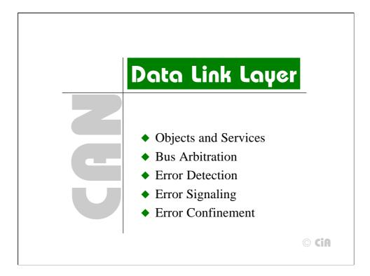
The CAN data link layer is standardized in ISO 11898. The data link layer services are implemented in the Logical Link Control (LLC) and Medium Access Control (MAC) sub-layers of a CAN controller. The LLC provides acceptance filtering, overload notification and recovery management. The MAC is responsible for data encapsulation (de-capsulation), frame coding (stuffing/de-stuffing), medium access management, error detection, error signaling, acknowledgement, and serialization (de-serialization).
