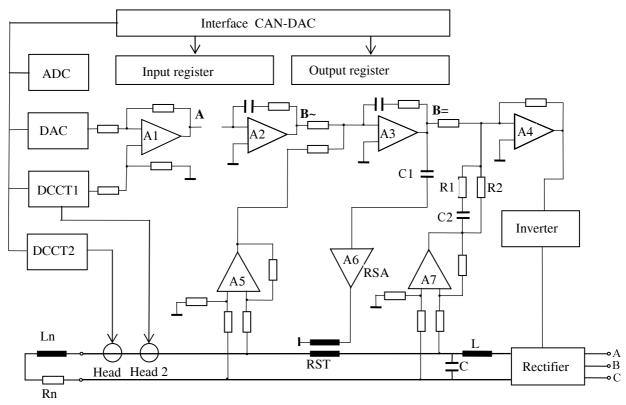
Figure 1: Simplified functional scheme of the Source.
