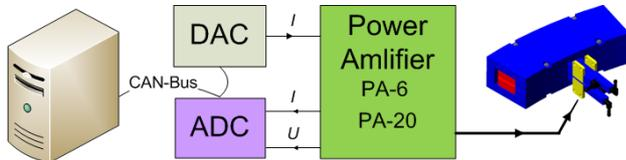
Figure 3: Steering coils supplying schematic.
