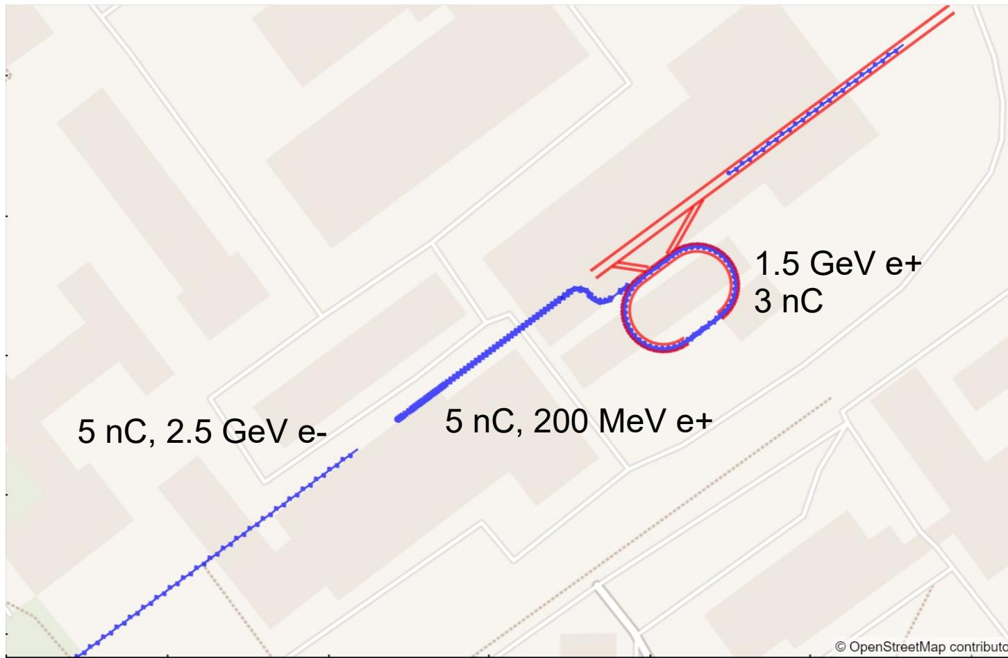
With 3.0 nC ( $2 \times 10^{10}$ ) e+ per shot it will take 10 Hz linac to get the required  $2 \times 10^{11}$  e+/sec. With 7 ms damping time we can have even faster linac, 20 Hz <sub>16</sub> operation will give a factor of two safety margin.
