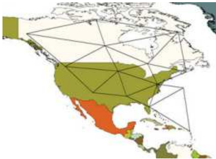
Figure 3.2: North American Satellite Triangulation Network [53]
