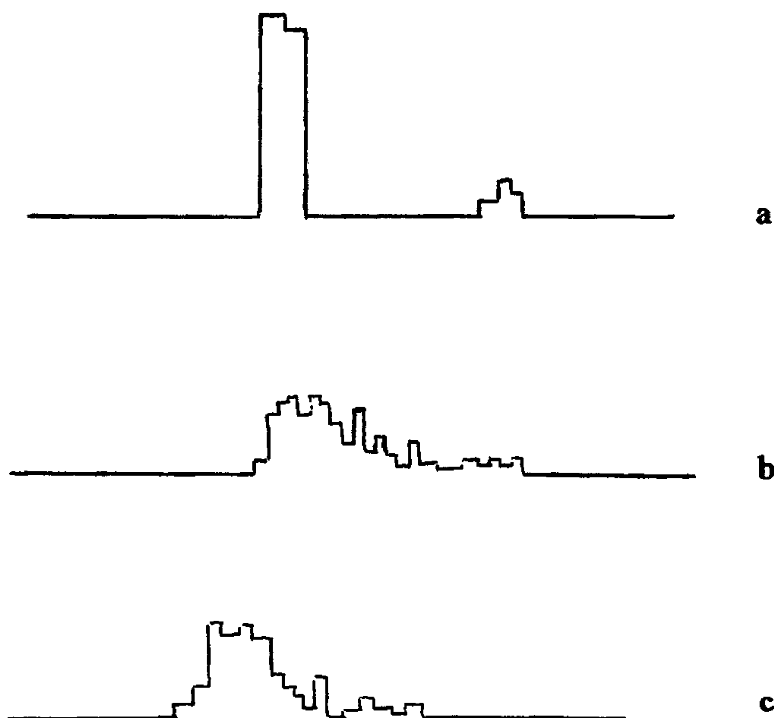
FIG. 7.18. The distortion of the beam momentum distribution by the injected beam; N=230 , \alpha=0.15 ; (a)—initial distribution, (b)—after 6 turns, (c)—after 12 turns.
