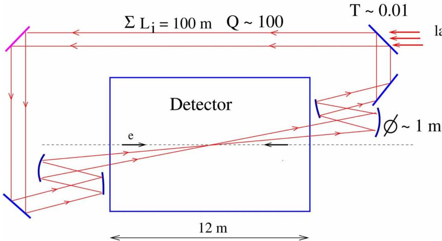
The cavity includes adaptive mirrors and diagnostics. Optimum angular divergence of the laser beam is  $\pm 30 \text{ mrad}$ ,  $A \approx 9 \text{ J}$  ( $k=1$ ),  $\sigma_t \approx 1.3 \text{ ps}$ ,  $\sigma_{x,L} \sim 7 \text{ }\mu\text{m}$
