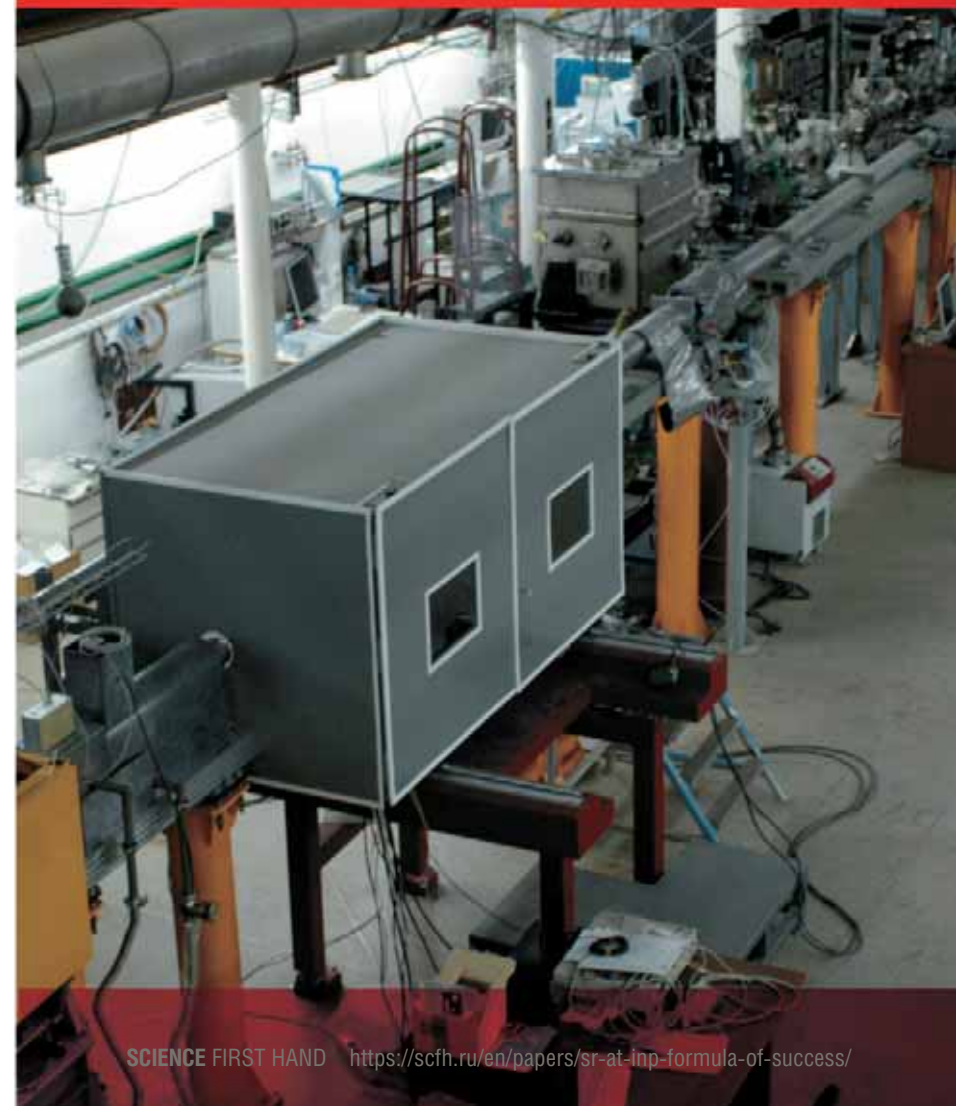
New station for studying detonation processes, planned for explosives weighing up to 200 g, in the VEPP-4 SR hall
