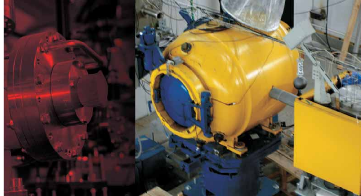
New station for studying detonation processes, planned for explosives weighing up to 200 g, in the VEPP-4 SR hall
