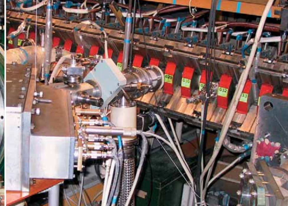
The multichannel analyzer of charge exchange neutrals measures the ion temperature of the order of 25 million degrees
