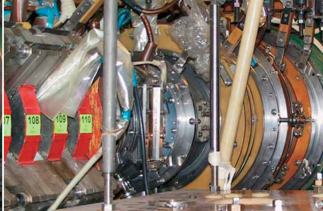
Experiments on studying the strength of materials under the action of a powerful plasma flow are performed in the output unit of the GOL-3 multimirror trap
