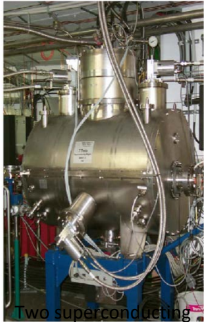
Two superconducting 7 Tesla shifters for BESSY-2 light source (Berlin). 2000,2001
