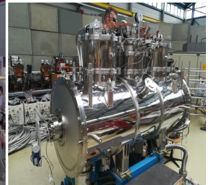
22-pole 7 Tesla, \lambda=125 mm superconducting wiggler for DELTA (Dortmund) 2019
