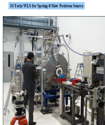
10 Tesla superconducting shifter for SPring-8. 2000
