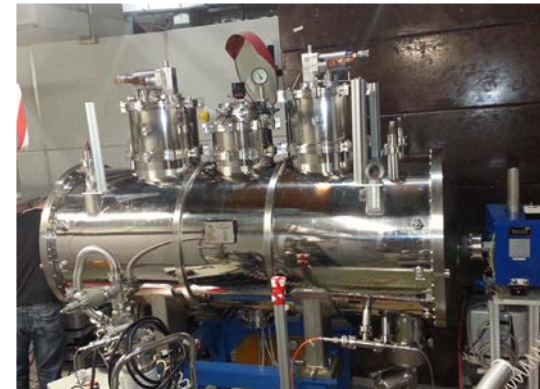
49-pole 3.5 Tesla, \lambda=60 mm superconducting wiggler for ELETTRA light source (Trieste) 2002
