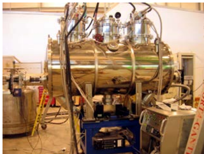
49-pole 3.5 Tesla, \lambda=60 mm superconducting wiggler for Diamond Light source. 2006
