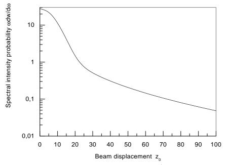
Figure 5: The spectral intensity probability  $\omega dw_{\gamma}/d\omega$  normalized to one particle in the beam in units  $2\alpha r_0^2 \Sigma_z \Sigma_y/\pi$  versus the vertical displacement of beams  $z_0$  (in nm).
