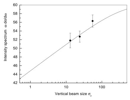
Figure 2: The bremsstrahlung intensity spectrum  $\omega d\sigma/d\omega$  in units  $2\alpha r_0^2$  versus the vertical sizes of beams  $\sigma_z$  (in  $\mu m$ ). The data taken from [6].
