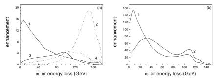
Figure 6: At settings of Fig.5; (a): probability and energy loss enhancements in silicon for SOS (1,2) and CB (3,4); (b): the same for SOS in diamond
