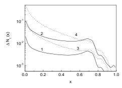
Figure 7: Number of photons per bin  $\Delta x=0.02$  in a diamond crystal at  $\varepsilon_0=250 GeV$  for CB ( 5 mrad off the < 001 >-axis and 160  $\mu$ rad off the (1 $\bar{1}$ 0)-plane) at L=0.1 cm (1) and L=0.5 cm (2); for SOS (325  $\mu$ rad off the < 110 >-axis in the (001)-plane) at L=0.04 cm (3) and L=0.2 cm (4);  $x=\omega/\varepsilon_0$ .
