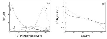
Figure 4: Yield from 1.5 cm-thick silicon crystal at (center of beam) settings as in Figs.2,3;(a): Power and energy loss spectra for SOS (1,2) and CB (3,4); (b): spectra (effective probabilities) for SOS (dotted) and CB (solid).
